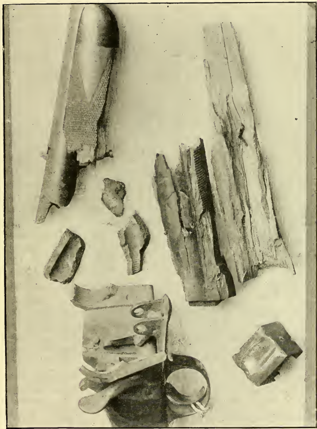
“Express” Rifle burst with Fine-Grain Powder.
